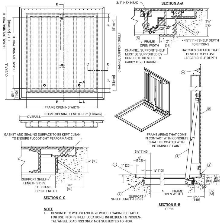
DESIGN FACTORY TESTED TO WITHSTAND 30' HEAD OF WATER 2.
