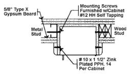
UL Classified 5/8" Type X gypsum board inserted in the cavity between the two lay-LISTED ers. Warnock Hersey has approved the Safeguard Cabinets to be mounted in any face of fire rated steel or wood stud for up to 2 hour rated walls without affecting its fire rating. The above meets the requirement test ASTM-E119-98 with test report WHI-495-1534. MOUNTING INSTRUC-TIONS are supplied with each safeguard cabinet.
